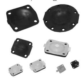
Diaphragms are molded in both the open and closed position dependent on type. All elastomer type diaphragms are attached to the compressor by a threaded stud. MPTFE diaphragms are attached by a bayonet type fixture that eliminates point loading, thus providing constant diaphragm compression across the weir resulting in a more uniform and reliable seal.
