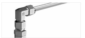
4. Connect union elbow to adapter by tightening SUPERLOK connection with wrench while holding elbow pointing in desired direction. Then insert tubing into the other end of the Union Elbow and connect tubing.
